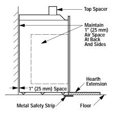
Note: Hearth extensions must not interfere with circulating grillwork
